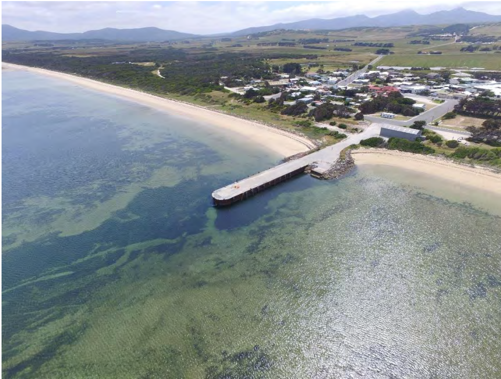
Figure 14 Aerial images of the proposed development site at Whitemark around the existing jetty, showing the shallow nature of the area and existing boat-track scouring.
