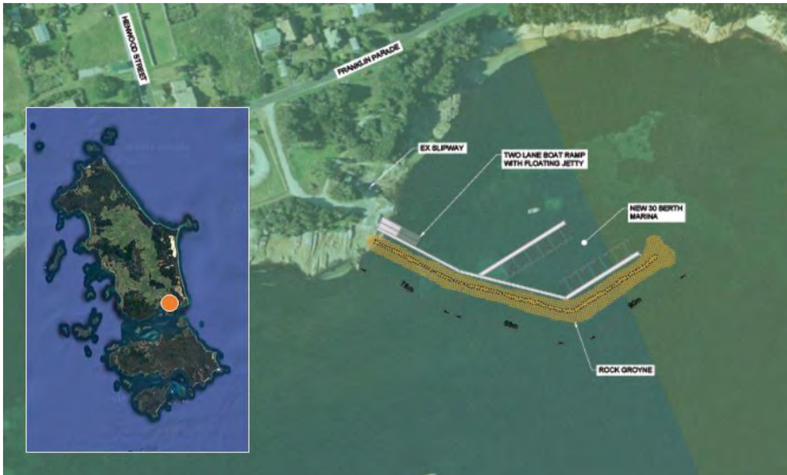
Figure 36 Map showing proposed development at Lady Barron Slip (inset image from LISTmap, 2016. Engineering design drawings from Burbury Consulting, 2016).
